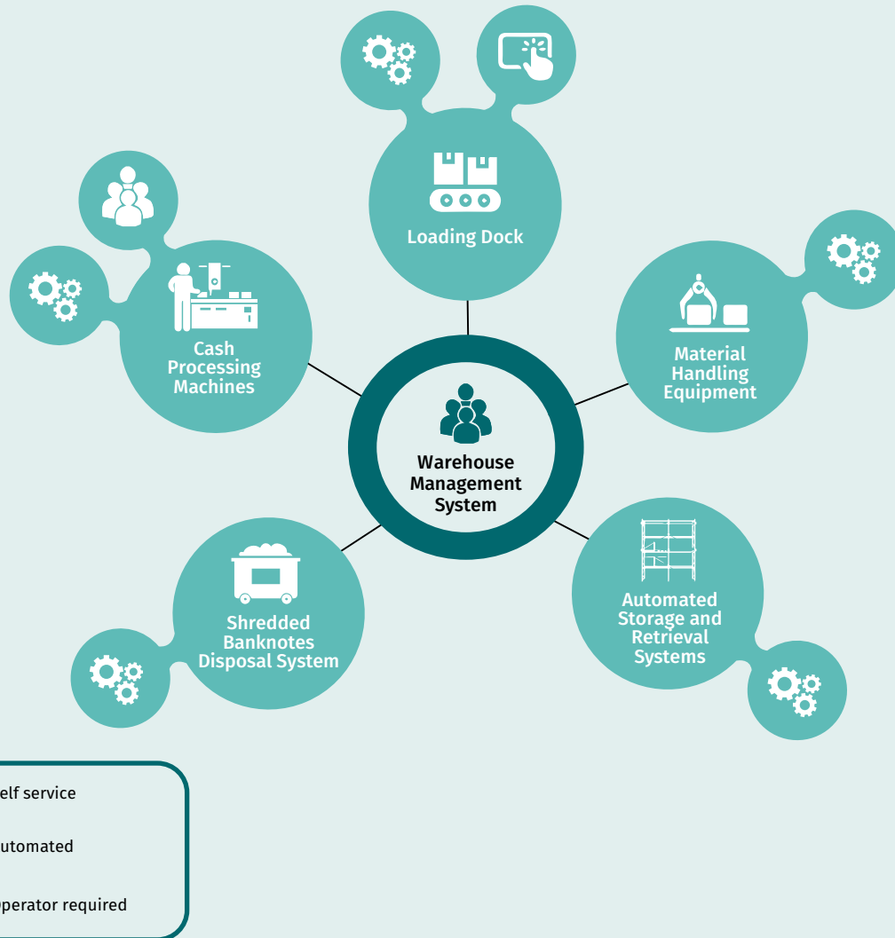
Diagram 2: WMS Central to the Automated Cash Operations at the ACC
