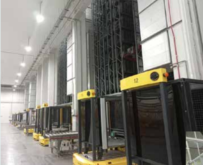
Movement of pallets of banknotes into and from the rack inside the vault managed by automated cranes.
