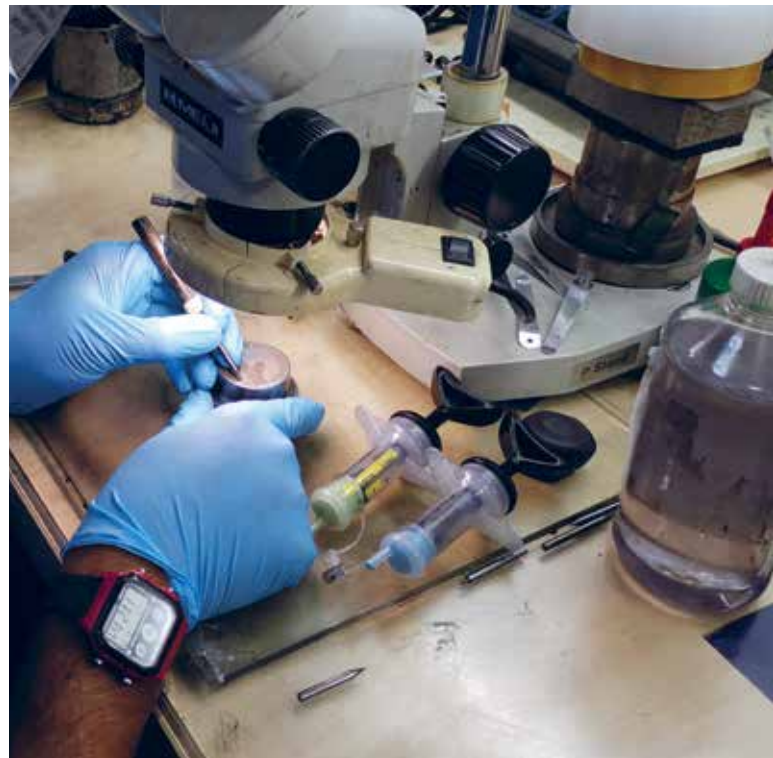
An engraver is applying the finishing touch on the master die as part of the process to mint commemorative coins.
