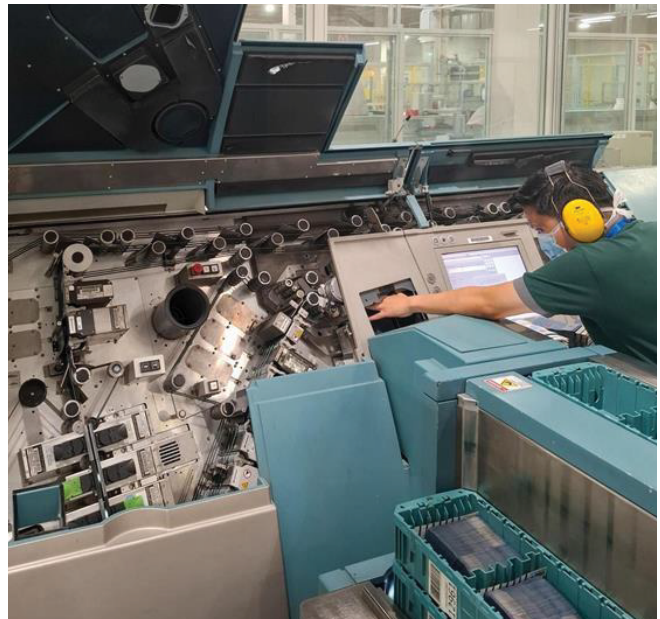
Unfit banknotes are detected by high-speed sorting equipment and withdrawn from circulation
