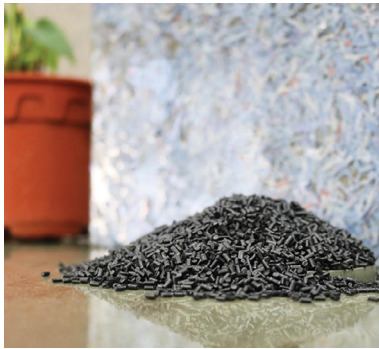
Shredded polymer banknote waste converted into polymer pellets can be used to make plastic products like flower pots and traffic cones, thus significantly reducing the need for virgin plastic.
